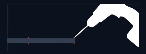
Using installation wire, beading wire, or fishing line, feed the wire from behind the housing/bezel, up and over the strip, then back down through the housing / bezel. Secure the strip by twisting the wire behind the housing or bezel.
