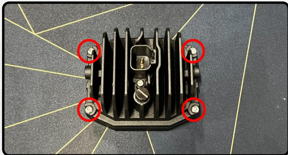
3. FLIP THE POD OVER AND REMOVE THE LENS HOLDER AND LENS. MAKE SURE THAT THE RUBBER LENS GASKET REMAINS IN THE LENS CHANNEL (GREEN), AND IS LAYING FLAT
