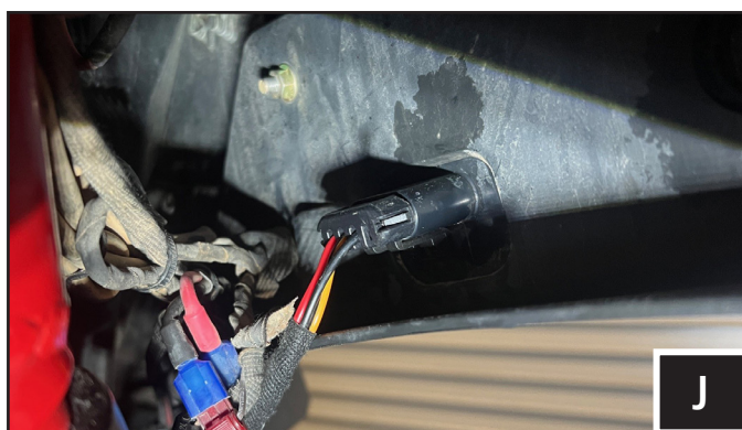
J. Run the "DRIVER OUTPUT" cable to the driver side tail light. Unplug the factory tail light connector and plug in the "DRIVER OUTPUT" connector of the RZR Rear Turn Signal Harness (B-H3112).
