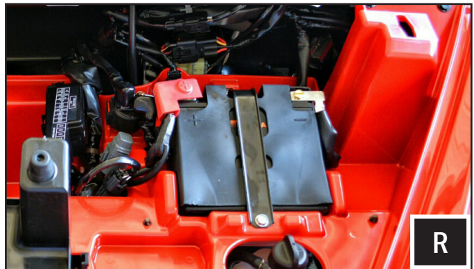
R. Run the BATT and GND wires of the Power Input Harness (B-H3413) to the battery and screw in the ring terminals to the.
