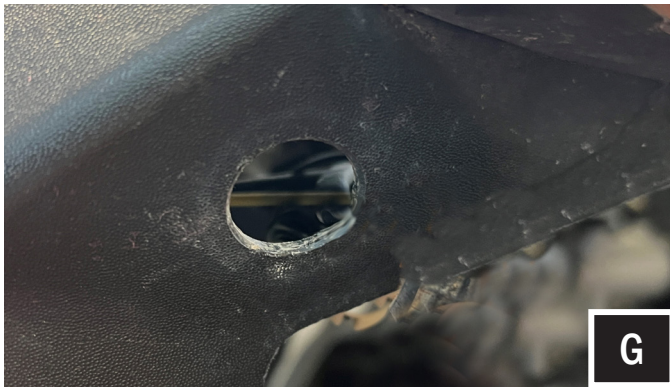
G. Drill a 3/4" hole in the front of the vehicle for the front turn signal LED lamp. Refer to the viewing angle diagram on page 6 for proper turn signal LED lamp placement.
