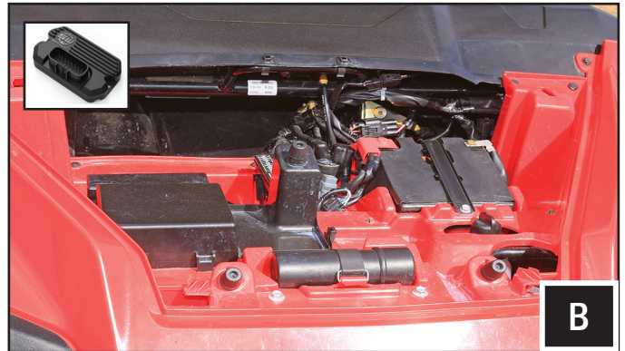
B. Lift and gently pull the dash cover away from the vehicle to expose the battery. Locate a suitable mounting location for the TANGO2 Turn Signal module. Secure the module to a panel using screws or zip tie it to a harness.
