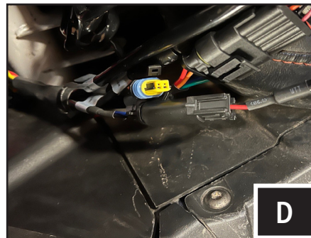
D. Plug in the controller cable, front turn signal extension cables (B-H2959) and rear turn signal harness (B-H3205) to the TANGO2 main harness (B-H3271).
