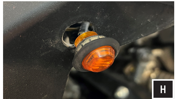
H. Insert the LED turn signal lamp into the hole and push in to lock in place. Repeat steps G and H for the other side.
