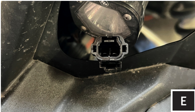
E. Route the front left and right turn signal extension cables to the front of the vehicle. Make sure to route the correct cable connector end that will plug to the LED lamp. Run the Horn power wires to the desired horn location.
