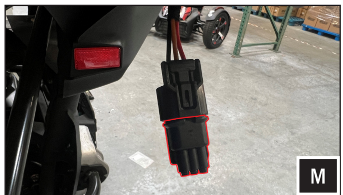
M. Run the "DRIVER OUTPUT" of the B-H3112 harness to the driver side tail light. Unplug the factory tail light connector and plug in the provided dummy plug to protect it from the elements.
