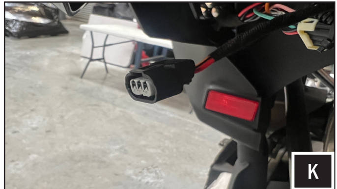
K. Run the KRX Rear Turn Signal Harness (B-H3112) to the rear of the vehicle. Begin installation on the passenger side tail light. Unplug the passenger tail light connector. See wiring image below for the passenger side connections.
