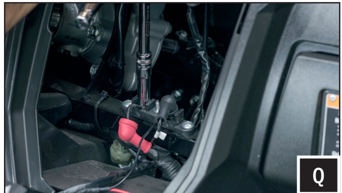
Q. Run the BATT, ACC and GND wires of the Power Input Harness (B-H3413) to the factory busbar and screw in the ring terminals to the corresponding battery, Accessory and Ground studs.
