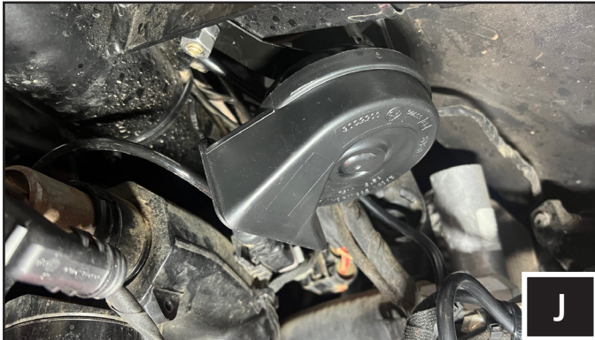
J. Horn mounting recommendations: 1. Mount away from moving parts; 2. Mount as high as possible; 3. Mount with the horn facing downward to protect from water damage.
