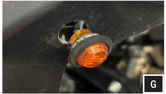
G. Insert the LED turn signal lamp into the hole and push in to lock in place. Repeat steps G and H for the other side.
