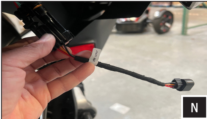
N. Plug in the KRX TS Adapter (B-H3122) to the B-H3112 “DRIVER OUTPUT” connector and plug the other end to the tail light. Use zip ties to secure the harnesses.
