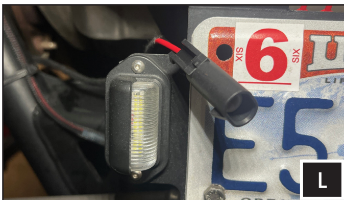
L. Run the "LIC. PLATE" connector towards the license plate location. Use zip ties to secure the cable away from any moving parts or the exhaust pipe.
