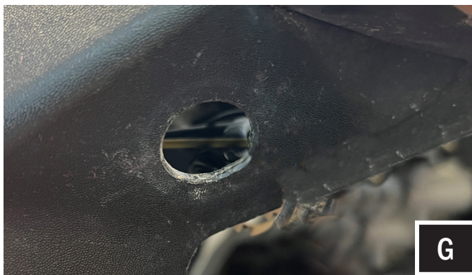
G. Drill a 3/4" hole in the front of the vehicle for the front turn signal LED lamp. Refer to the viewing angle diagram on page 7 for proper turn signal LED lamp placement.
