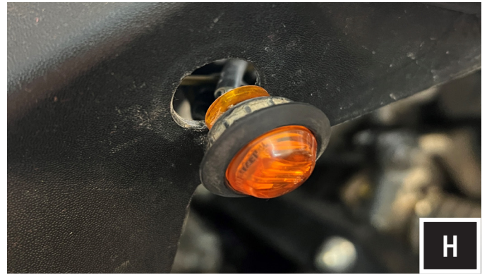
H. Insert the LED turn signal lamp into the hole and push in to lock in place. Repeat steps G and H for the other side.
