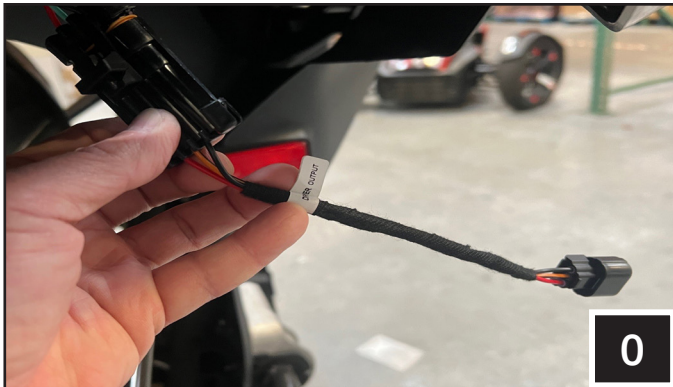
O. Plug in the Defender TS Adapter (B-H3122) to the B-H3112 "DRIVER OUTPUT" connector and plug the other end to the tail light. Use zip ties to secure the harnesses.
