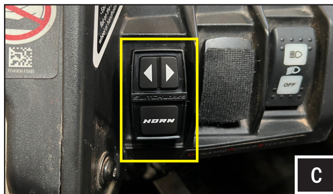
C. Use a vacant rocker switch mounting slot and insert the TANGO2 turn signal rocker switch. Run the cable towards the TANGO2 brain module.
