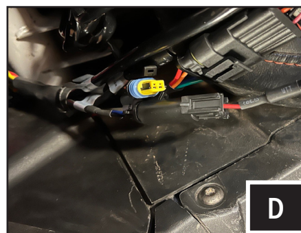
D. Plug in the controller cable, front turn signal extension cables (B-H2959) and rear turn signal harness (B-H3112) to the TANGO2 main harness (B-H3271).
