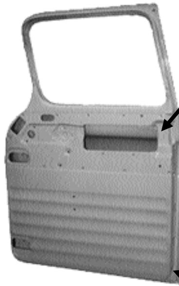
Access hole in door, used when marking the glass on the window sash.
