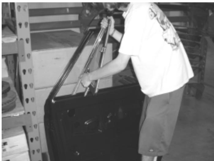
**(2)** Remove the complete vent window assembly by unscrewing it from the door. There are be three screws at the top, front edge of the vent window (**Picture A**) & two retaining bolts at the front, bottom of the door (**Picture B**). May require some manipulating in order to remove the vent window assembly, it is a tight fit.
