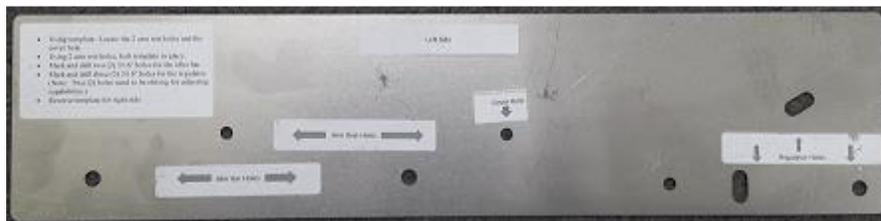
Before putting the window regulator in, you will need to install the front channel guide. With this guide, you will also need to drill on the front edge of the door. Drill a 5/16" hole 2 inches down from the door panel and 2-3/4" from the inside edge of the door.
