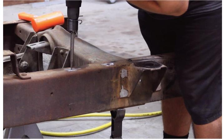
Now that BOTH sides have been drilled, cut-off and the bed and cab mounts have been removed, it's time to relocate the cab mounts. You'll be using the center section of the template that was set aside earlier, but first the Template needs to be prepped.
