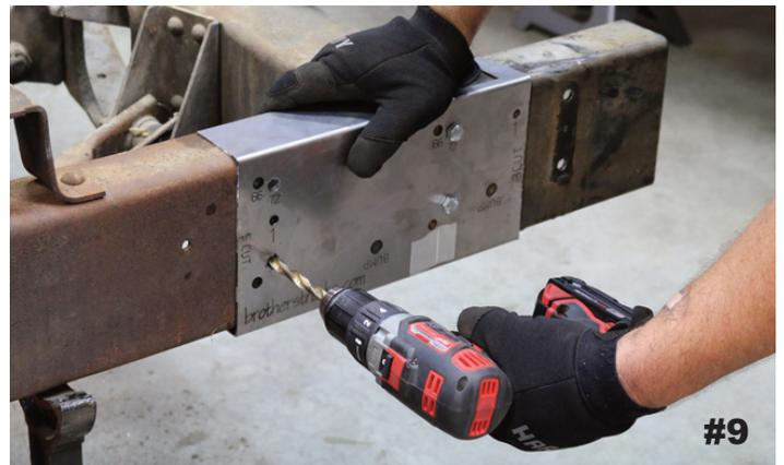
\* With the Template in place, using a 1/8" drill bit, drill the NON-underlined holes that correspond with your year range (72 for '67-'72, 66 for '63-'66) as shown above in #9 on a 67-72 frame.
