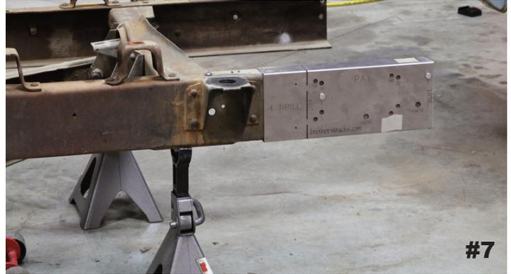
**Template Step 4.** Drill all holes in the panel marked **4 DRILL** on the template using a 1/8" drill bit. Do this for BOTH the DR and PA sides before moving on to Step 5. There are 2 holes on the face of this panel, and 1 additional hole on the top and bottom (total of four 1/8" holes per side).
