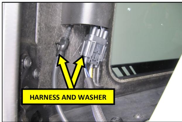
13. Reconnect the wiring harness and washer fluid line.
