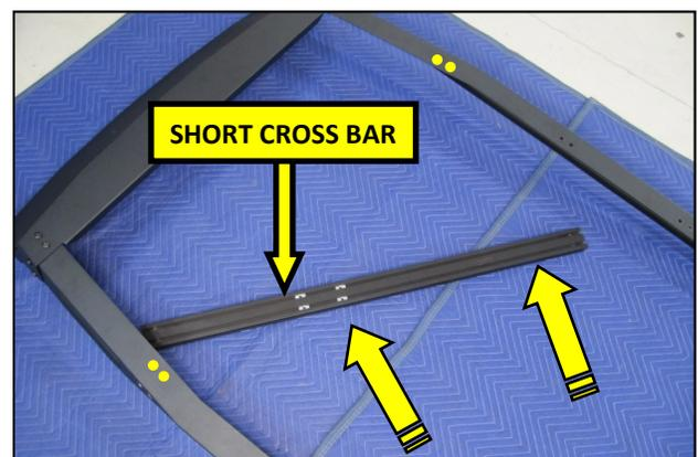
25. Slide the Short Cross Bar between the Rails and align it with the first set of holes in the Rails.
