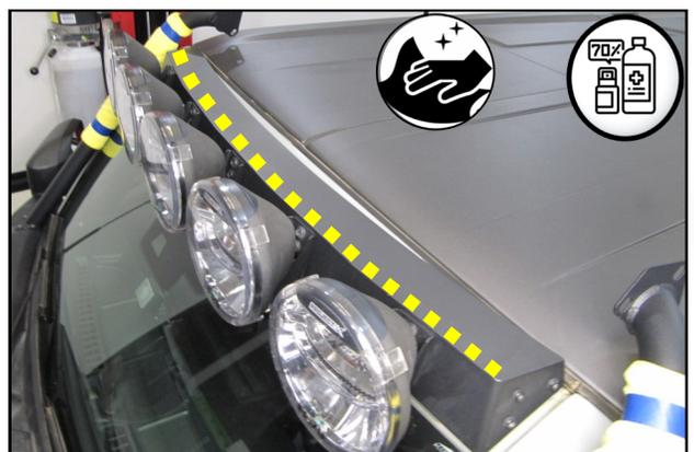
37. Clean the leading edge of the light bar using a mild solution of soapy water, followed by isopropyl alcohol.
