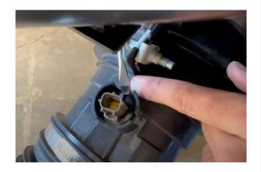
Clip in the IAT extension harness, then zip tie the harness to the side on the engine bay as shown in the picture.
