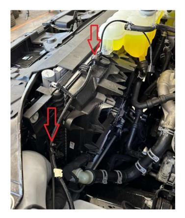
Install the IAT grommet onto the S&B intake tube.
