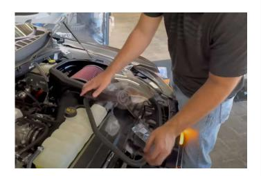
Snap the assembled S&B clear lid onto the airbox.
