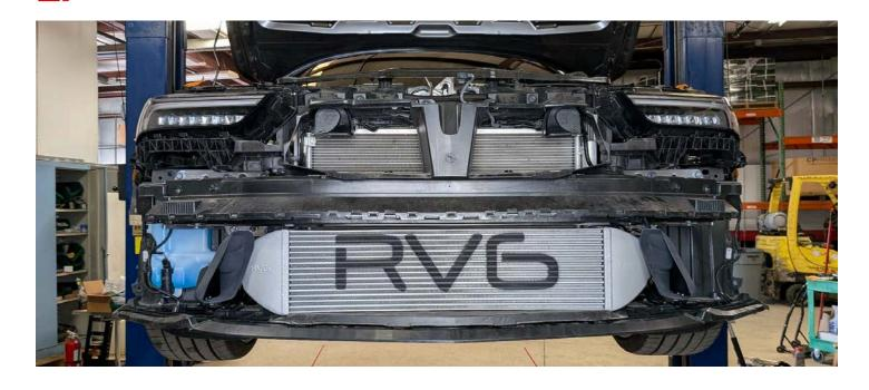
**NOTE:** The push-pins do not need to be re-installed in the location circled in red. The Intercooler will be sitting on top of the bottom guard, there won't be enough clearance for the push-pins to lock into place.
