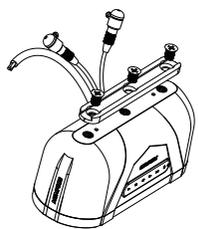
Attach bracket to desired mounting location using provided screws
