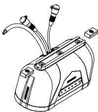
Slide mounting points into the channel
