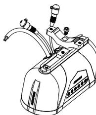
Screw UTV bracket into threaded mounting points
