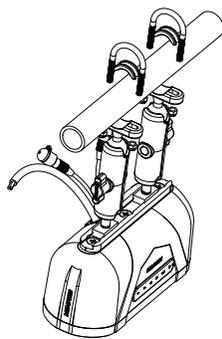
Use appropriate U bolt to connect the MXASB9 to the bar
