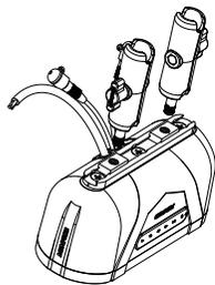
Screw mounting posts into threaded mounting points
