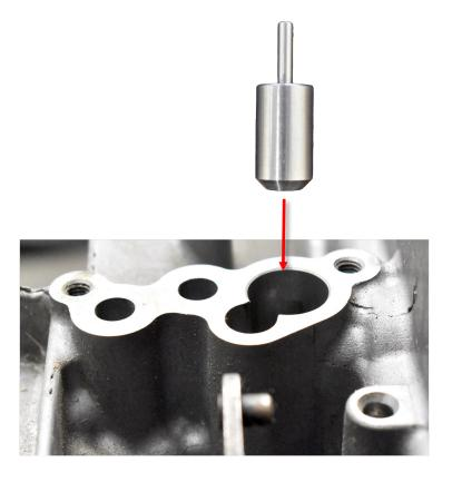
**2.** Install new Cooler Bypass Valve with pin pointing up.
