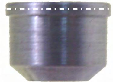
**2nd type capsule only:** Grind the head of the new capsule to the dashed line. **Clean grinding flash from orifice hole.**
