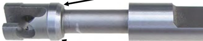
Grind 1/16" to 3/32" (.063 to .096) Chamfer Here.
