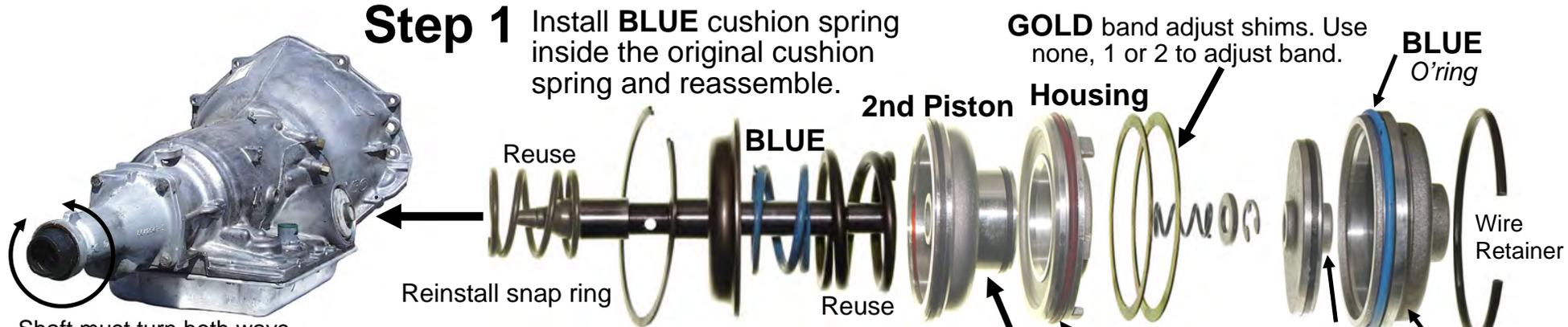
**Step 1** Install **BLUE** cushion spring inside the original cushion spring and reassemble.
