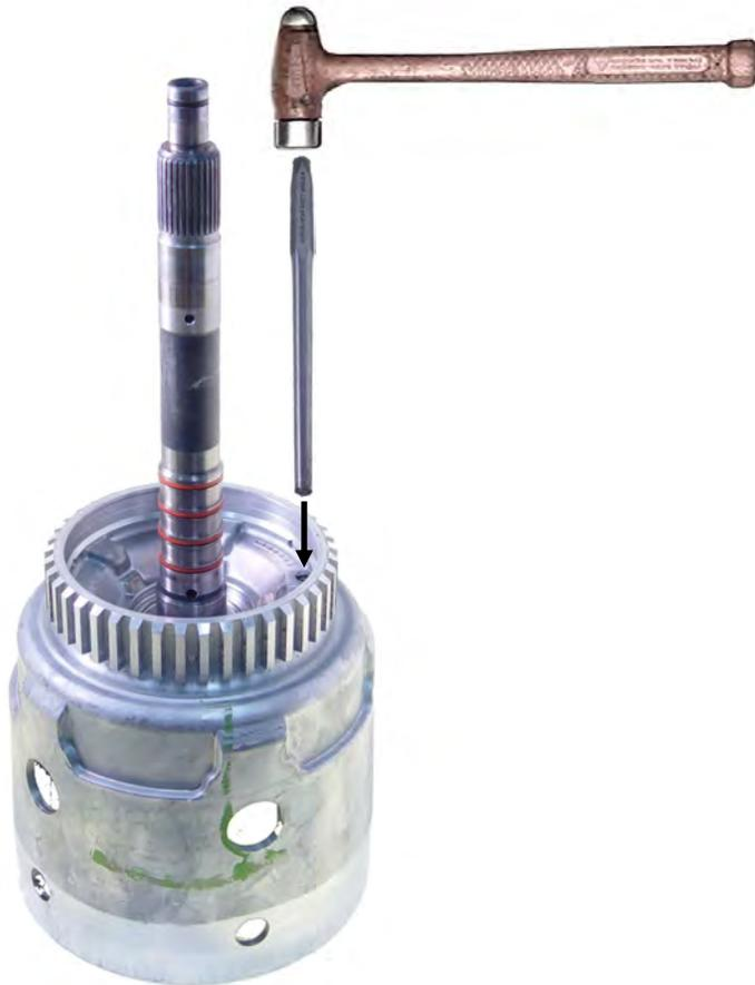
**After orifice is installed 3-4 piston should not rock when placed in drum.**
