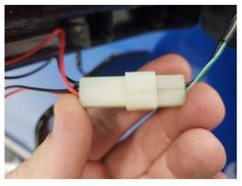
**Step 5\\**Connect the new Axial mirror light harness to the factory mirror light harness.
