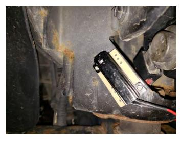
**Step 4\\**Mount the resistor to the frame using the supplied adhesive. \*\*Note: The ballast will get hot. Keep away from anything that may cause damage.
