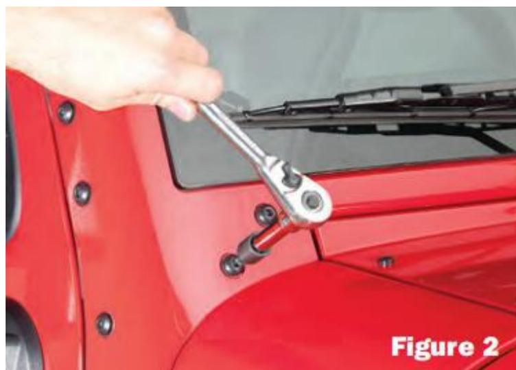
3. Position the Bracket. Position the passenger side windshield light bracket pre-drilled holes over the holes left from removing the torx screws. They should line up exactly.
