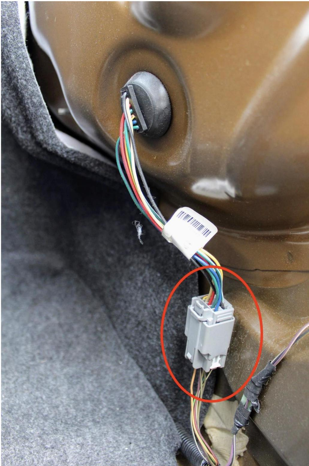
8) Push the rubber grommet through the hole (1 on each side) using your finger.
