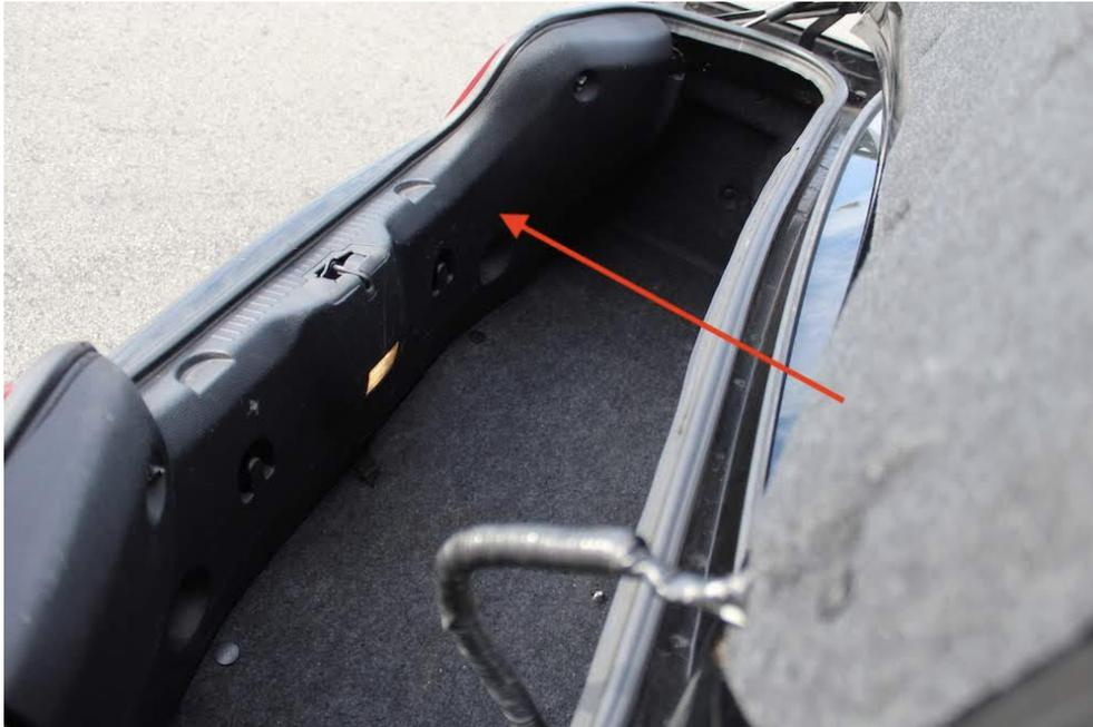
**2)** Remove the 2 twist off nuts (1 on drivers side, 1 on passenger side) simply by twisting them off with your hands.
