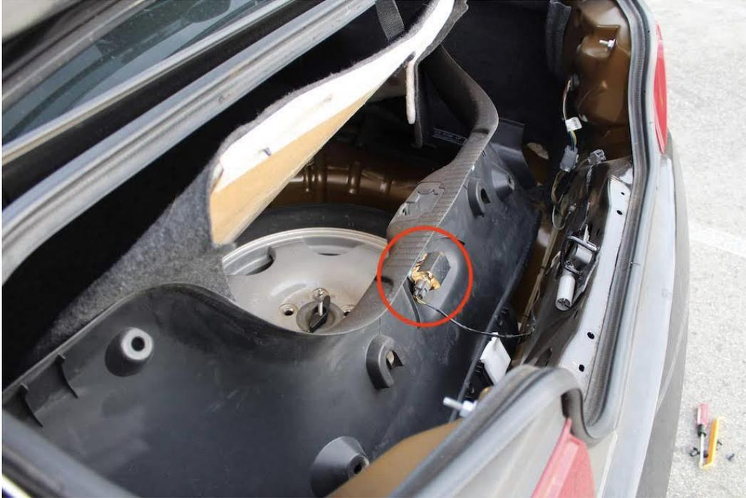
5) Remove (1) 13mm bolt found in the corner of the trunk near the tail lights. It is at the top on each side.
