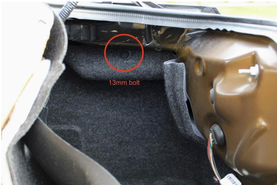
6) This should allow you to pull back the soft trunk lining. It will expose (3) 11mm nuts that you can remove to unbolt the taillight. There are 3 nuts on each side.
