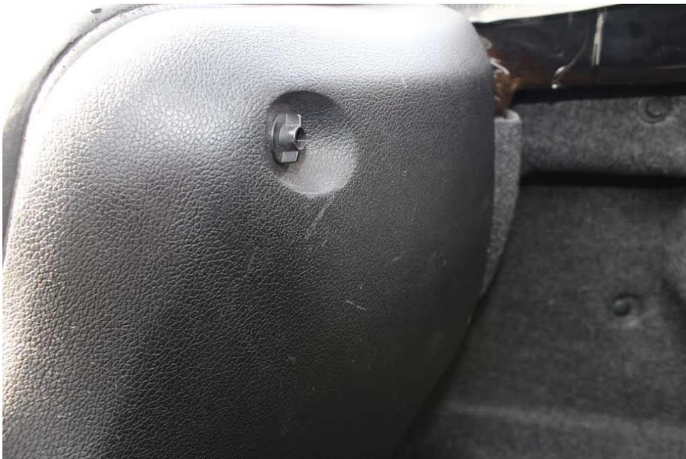
3) Remove the 2 interior trim plastic screws (1 on driver side, 1 on passenger side) by using a flathead screwdriver or an Interior Trim Remover tool.
