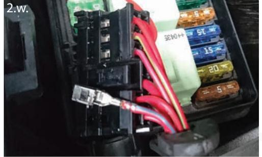
2.x. Solder the orange wire from the supplied pump loom to the pin as per image. Reinstall the pin into the connector, refit the plastic locking clip and insert connector back into the fuse box.
