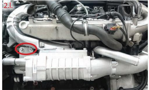
2.m. Cut the original breather tube about 30mm towards the right of the image (red line) and fit the newly pulled through rubber hose as per the image over the end of it.
