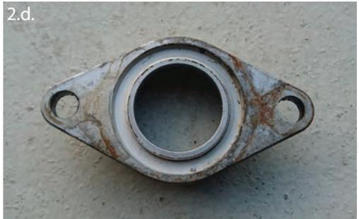
2.e. Fit the O ring from this flange into the flange on the new outlet pipe supplied and screw it back onto the block, ensure sealing face is cleaned on the block first.
