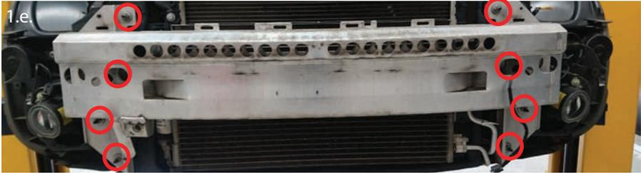
1.f. Remove the lower outer crash beams that connect to the sub frame by undoing the two large bolts located on the underside of the vehicle and the M6 screw that fixes into the radiator support panel from the front.
