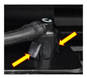
6. Push the nozzles into the appropriate holes on the Forge Motorsport water spray bracket, making sure to copy the same orientation (nozzle spray on underside of bracket, water line on top side of bracket)
