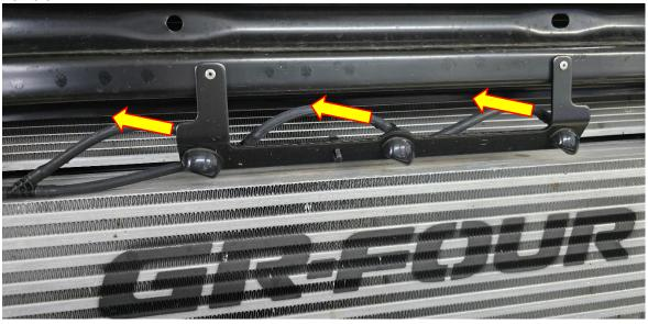
2. With the crash bar removed take your drill with a 3.5mm drill bit inserted and carefully drill out the two rivets that hold the OEM water spray bracket in place. Once the rivets are removed use a 7mm drill bit to increase the size of the drilled hole, this will be required for the rubber riv nut which will now be used to hold the Forge Motorsport water spray bracket in place.
