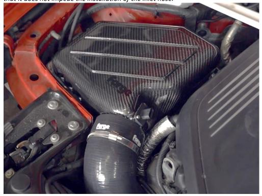
**11**. With the inlet hose secured you can now use the four latches from the OEM lower airbox to secure FMINDK55 in place.
