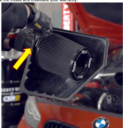
9. FMINDK55 fits to the lower airbox in the exact same way that the OEM upper airbox fits. Place it onto the lower air box but do not latch it down yet.
