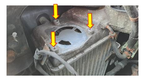
5. With the rubber o-ring facing down, place the Forge spacer plate in position
