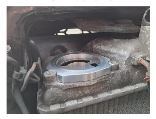
6. Place the Forge Motorsport valve on top of the spacer plate, align the 3 holes and bolt in position using the supplied bolts and washers.
