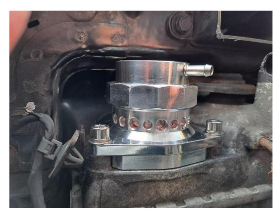
7. Using pliers either re-attach the OEM vacuum line to the Forge Motorsport valve, or replace it with the supplied vacuum line.
