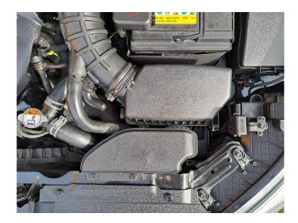
2. Unclamp and remove both the small vacuum hose and large recirculation hose.
