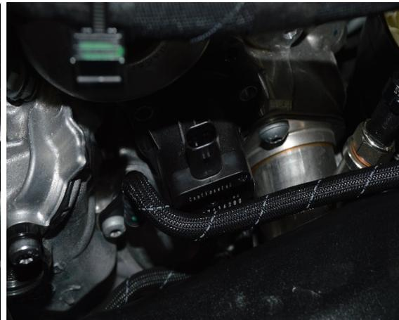
9. Ensure the supplied O-rings are in place on the base of the Forge Motorsport valves then attach the valves into the mounting position taking note that the valves are handed for the left and right hand turbo, this is to avoid interference with the turbos actuators. Use the removed torx fasteners on each valve to secure them into position.
