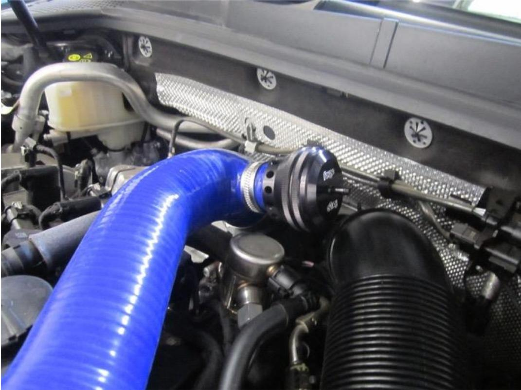
12. Push the Forge vacuum T over the vacuum port on the inlet manifold, secure it with the E-clip provided and reconnect the OEM vacuum hose (removed in Step 2.) to the other side of the Forge vacuum T.
