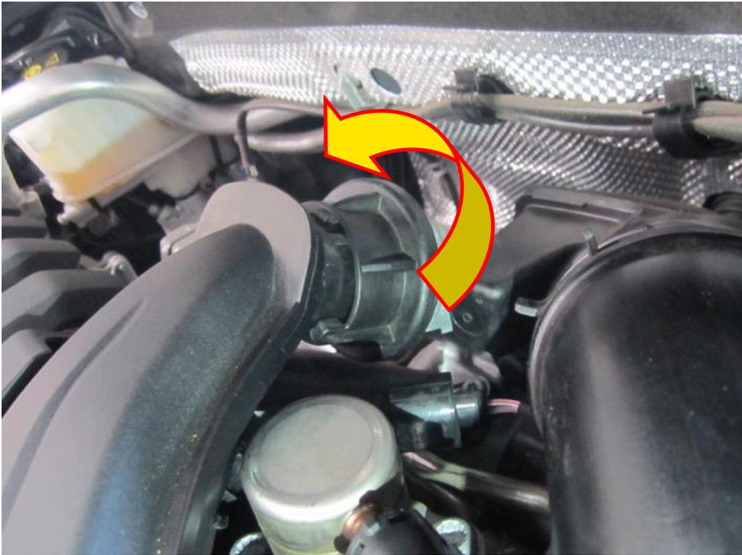
4. With the use of a flat blade screwdriver or trim tool, release the plastic retaining clip which holds the other end of the boost inlet pipe. The boost pipe will now be free at both ends and will pull away from the engine bay.
