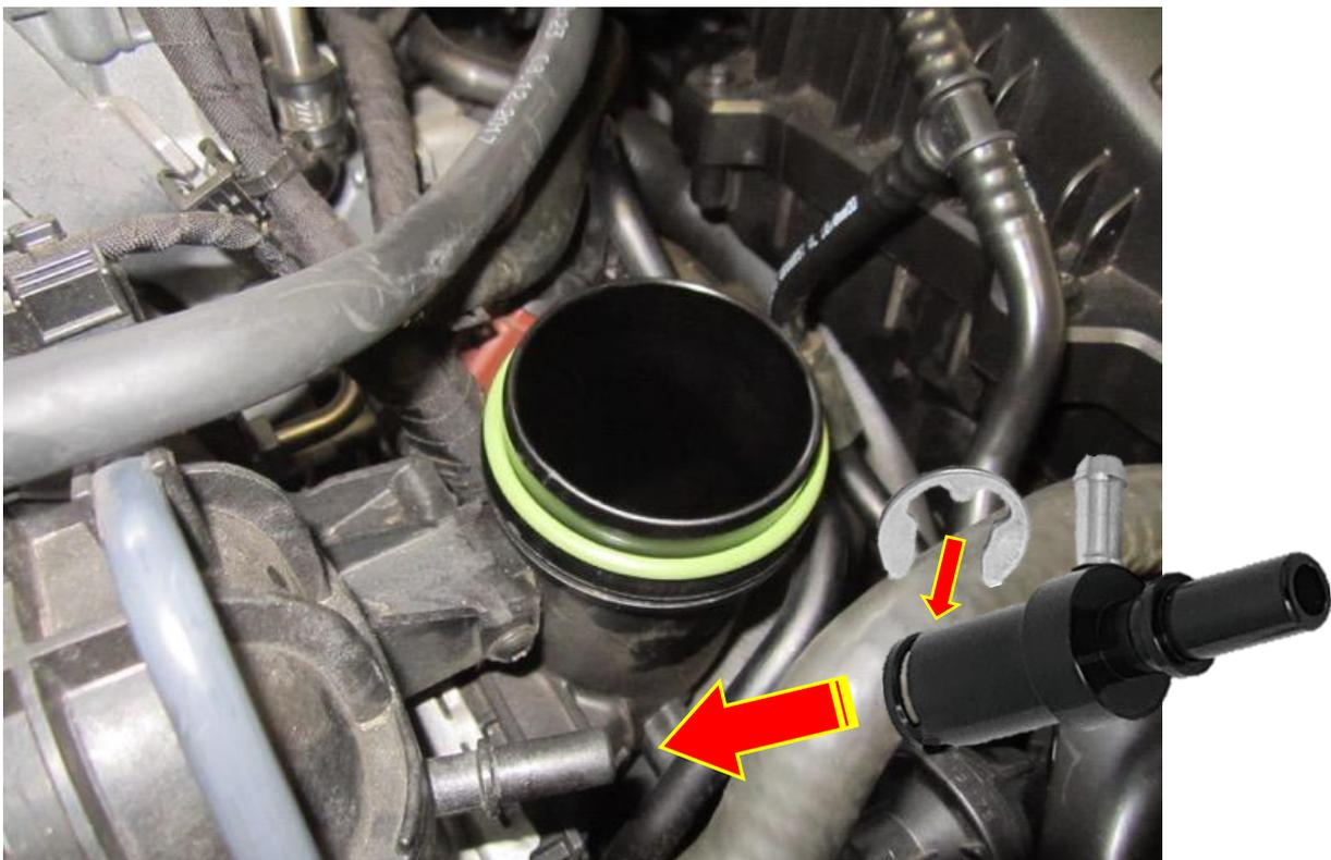
13. Push one end of the supplied silicone vacuum hose onto the Forge vacuum T and secure it with a cable tie. Run the vacuum hose up to the dump valve and cut to length with scissors or a sharp knife. Use cable ties provided to route it away from any moving parts.
