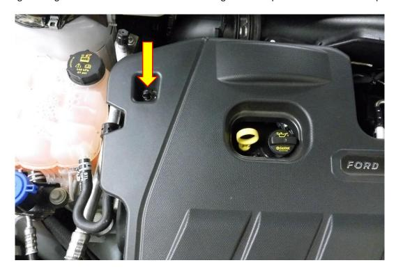
2. Remove the vacuum pipe located at the front of the inlet manifold. Push the green button inward and pull the pipe away at the same time, this will allow the vacuum pipe to come away.
