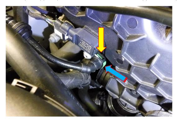
3. Take the supplied vacuum T piece adaptor and insert the smaller end into the vacuum pipe removed in the previous step. Now re fit the vacuum hose and adaptor back into place, once pushed as far as it will go, lock into position with the supplied retaining clip.
