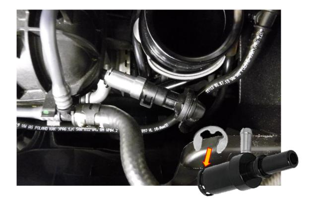
4. Push one end of the supplied silicone vacuum hose onto the Forge vacuum T and secure it with a cable tie. Run the vacuum hose to the part you are adding and cut to length with scissors or a sharp knife. Use cable ties provided to route it away from any moving parts.
