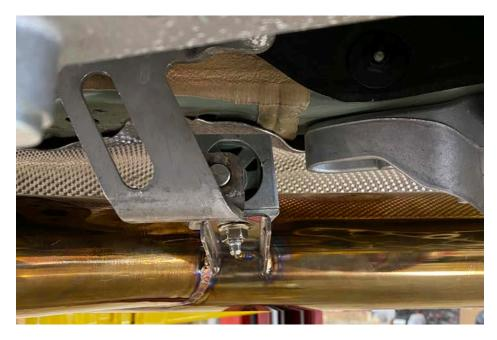
• All clamps and hanger bolts point straight down to make sure no point on the system will catch on anything.
