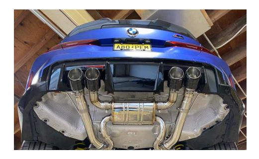
6. Install the new Valvetronic Designs axle back system by lifting the system into place and <u>loosely</u> installing the exhaust hangers by the rear diff and rear bumper.
