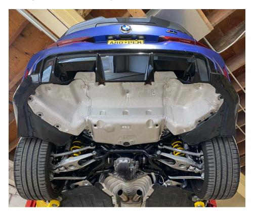
5. With the stock system and the Valvetronic Designs system on the ground, move the rubber exhaust hangers and valve control motors over to the new system.
