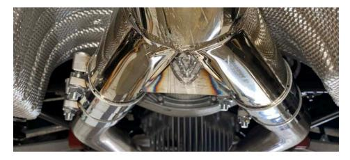
• Valvetronic Designs logo is "right side up" as in not "upside down" where the Y-pipe connects to the rear section.
