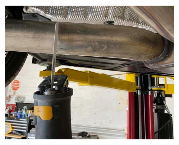
1. Loosen and lower, but do not fully remove the exhaust hangers by the rear diff. This will give you more room to cut the midpipe from the axle back unit between the 2nd and 3rd dimple. File down any burrs.
