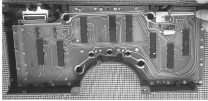
4. Remove the twenty-two (22) 7/32" screws securing the Display Driver Board of the gauge unit.
