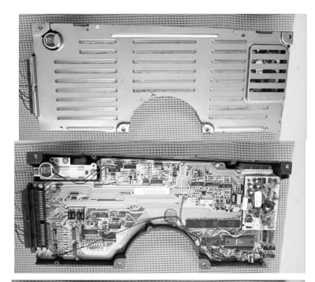
3. Remove the seven (7) 7/32" screws holding the Logic Board to the gauge unit.
