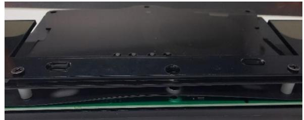
4. Attach the acrylic lens panel using 2 1 ¼" screws with 3/8" spacers at the top of the lens and the 1 ½" screws with ¾" spacer at the bottom of the panel as demonstrated in the above pictures. Secure all screws with a nylon washer and locking nut on the back of the assembly.
