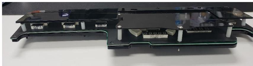
5. Mount the completed assembly back into the original stock bezel using the five (5) thread forming screws provided.
