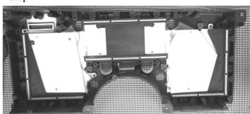
Remove the twenty-two (22) 7/32" screws securing the Display Driver Board of the gauge unit.
