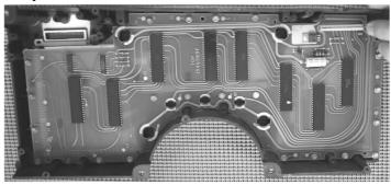
Remove the six(6) 7/32" screws securing the back panel.
