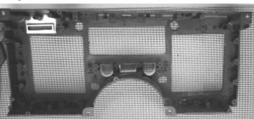
Remove the six (6) rubber clips securing the lenses.
