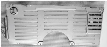
Remove the factory LED gauge unit from the dash panel.
