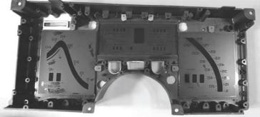
Remove the stencils and rubber blocks from the edges of the LED displays.
