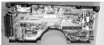
Remove the seven (7) 7/32" screws holding the Logic Board to the gauge unit.
