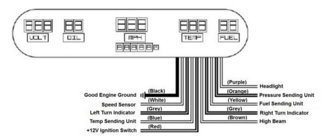
Ground - **Black** This is the main ground for the display system. A wire should be run from this board to the vehicle's main engine block ground. Use 18 AWG or larger wire to ensure sufficient grounding. Proper vehicle grounding is extremely important for any gauges (or electronics) to
