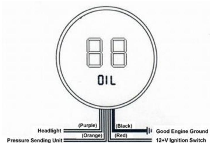
*Ground - **Black** Connect directly to an engine ground such as the engine block. For the most accurate readings, connect to the same ground as that to which the sending unit is attached.*
