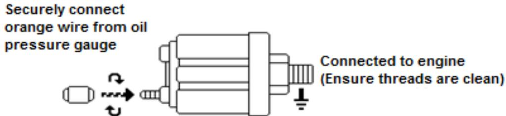
**Make sure** that the connection between the oil pressure sensor and the engine is clean and **does not** have Teflon tape or any other sealants on the threads. This provides a stable ground for the sensor which will not function if it is inhibited.
