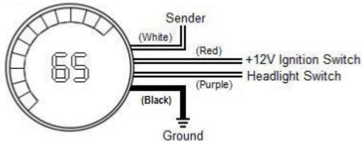
**Power – Red** Connect to a switched +12V source (such as the ignition switch)
