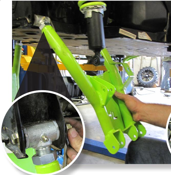
Install the new LOWER control arm to the frame, using the factory hardware. (17mm)
