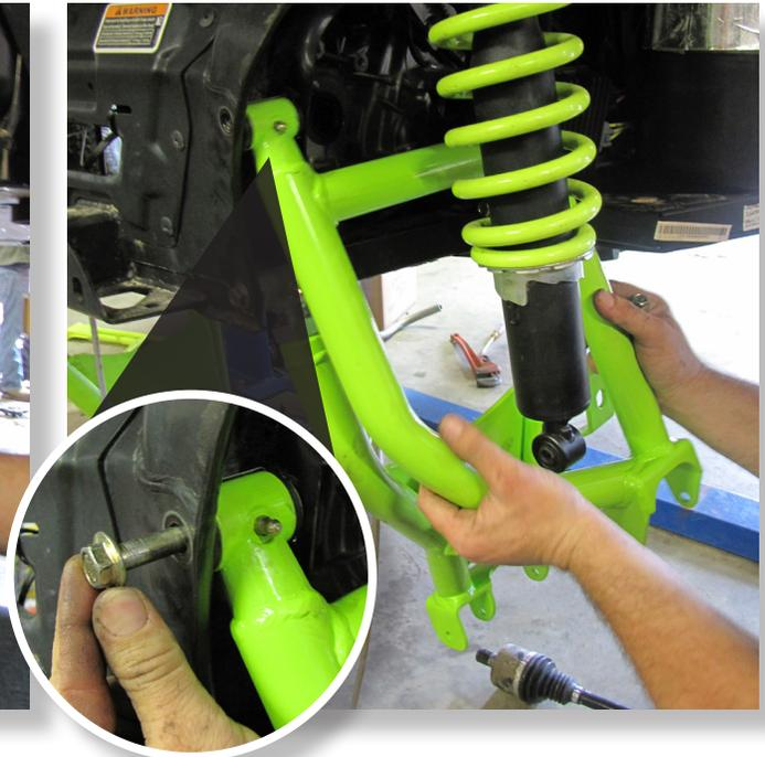
Install the new UPPER control arm to the frame, using the factory hardware. (17mm)
