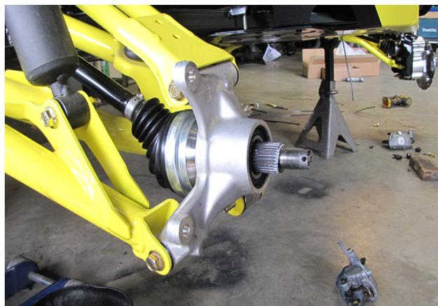
Remove the bolts and nuts that attach the rear knuckle to the upper & lower A-arms. (15mm) **KEEP FACTORY HARDWARE.**
