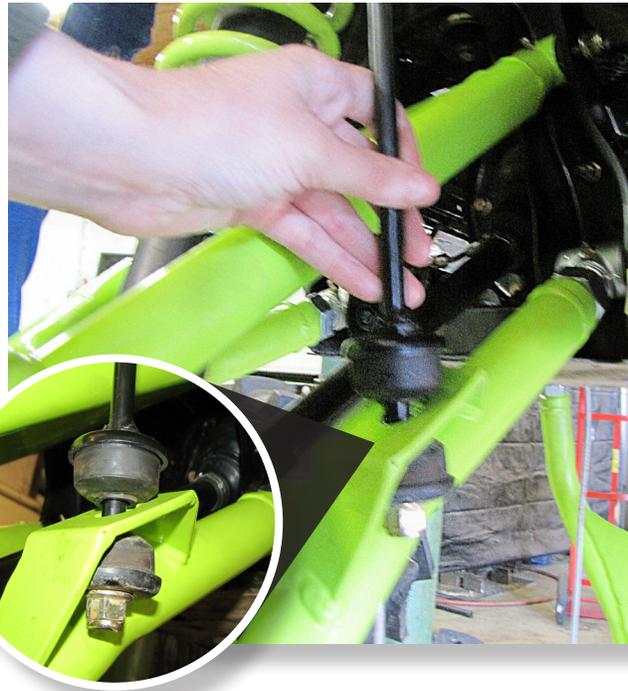
Secure the sway-bar link to the sway bar tab on the **LOWER** arm by re-securing the linkage bushing.
