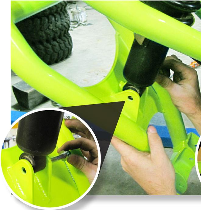
Secure the shock to the **LOWER** arm by installing a **M10x55mm** bolt followed by a **10mm** washer through the shock tab. Secure it with another **10mm** washer and **10mm** lock nut.
