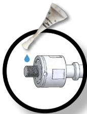
Lightly apply blue loctite to the inner tie rod, where it connects to the rack and pinion.
