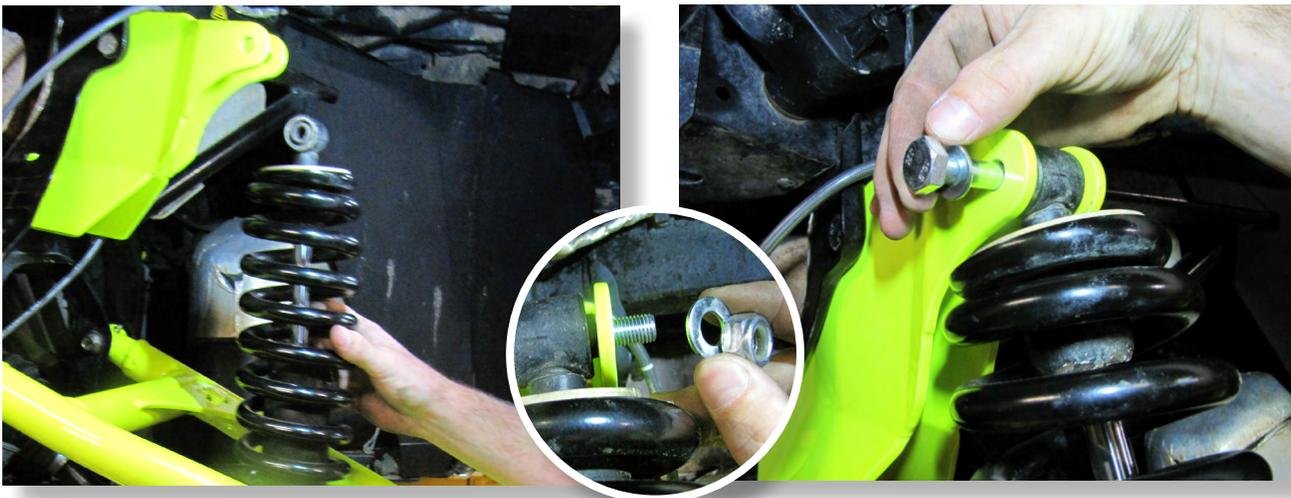
**Install the shock at the rear lift bracket.**
