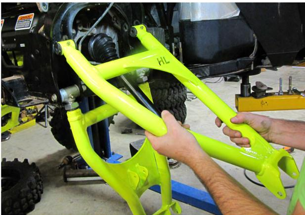
Connect the new upper arm (134U) at the frame using the factory hardware.
