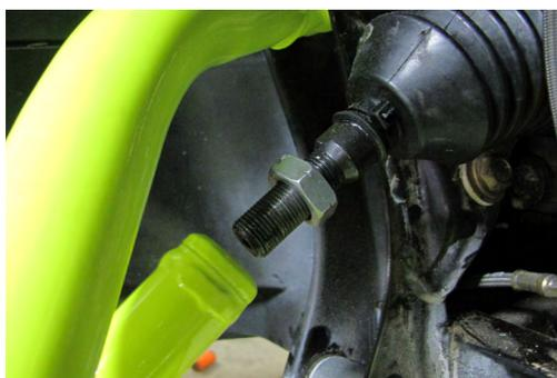
You will need to turn the steering wheel closer to the center to allow play in the boot. Slide the boot back down and secure it with an 11" zip tie.
