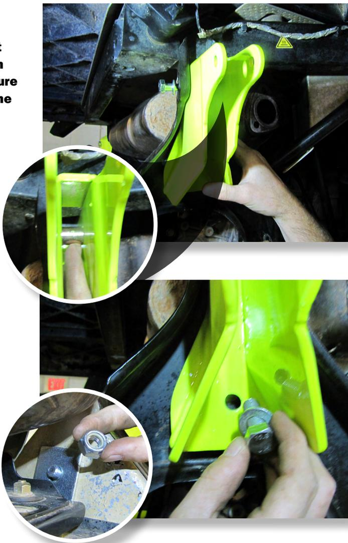
Secure the lower portion of the lift bracket with the 12x30mm bolt followed by a 12mm washer.
