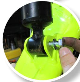
Use a 10X55 bolt followed by a 10mm washer to secure the **LOWER** shock to the lift bracket. Secure bolt with 10mm washer and 10mm lock nut.
