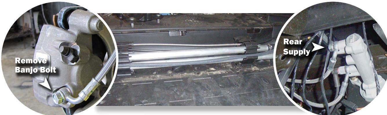
Disconnect the rear brake lines from the calipers. Have a container ready to collect fluid. Disconnect the rear supply line from the cylinder then remove it and the factory REAR brake lines. It is faster to cut the lines since they will not be reused, but is not necessary.
