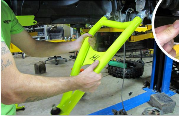
Install the new lower control arm to the frame, using the factory hardware.
