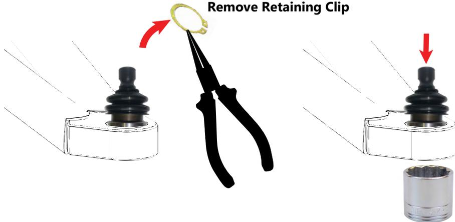
Back the ball joint with a large 36mm socket or something sturdy of similar diameter, then using a press or vice, press the ball joint out of the arm.
