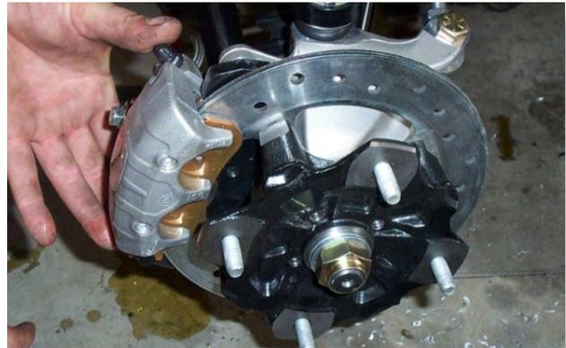
Connect the caliper to the hub assembly.
