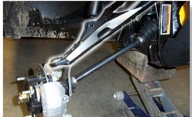
Disconnect the Upper arm by removing the bolts at the knuckle, sway bar, shock, and the frame. **KEEP ALL FACTORY HARDWARE.**
