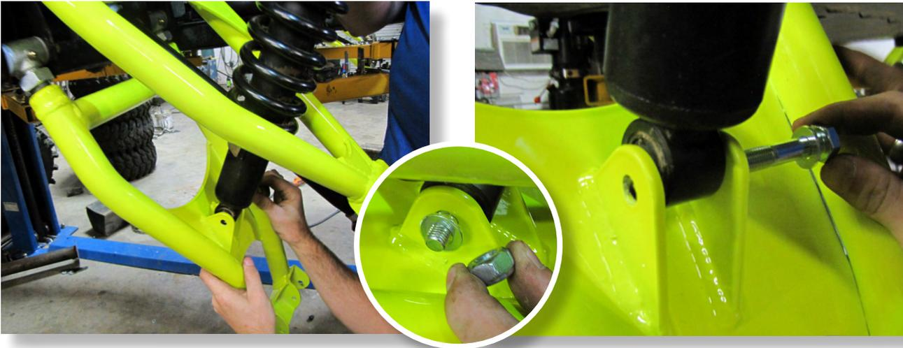
**Install the shock to the lower arm shock tab.**
