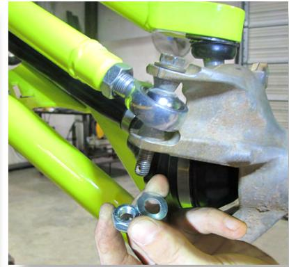
Secure tie rod bolt with a 10mm washer and 10mm lock nut.
