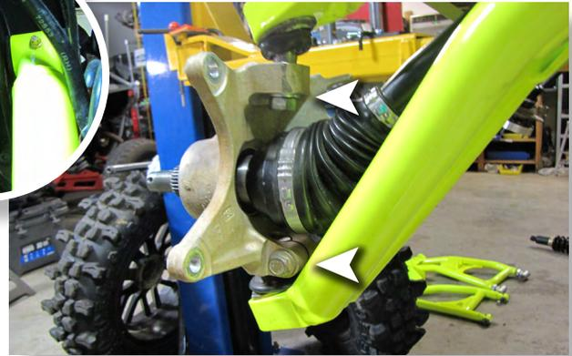
Secure the arms to the knuckle at the pinch bolt and the lock nut on the upper portion of the knuckle. Install cotter pin.
