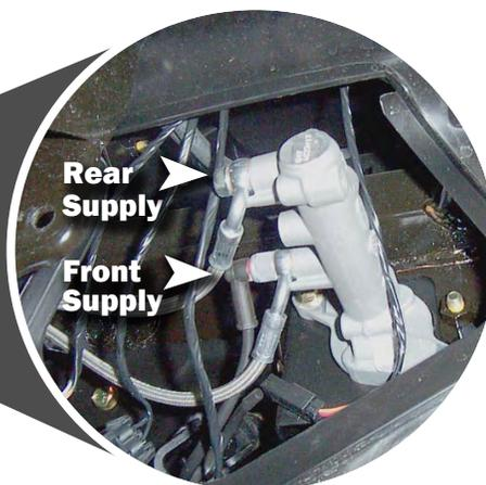
Disconnect and remove the factory FRONT SUPPLY LINE. Have a container ready to collect fluid.
