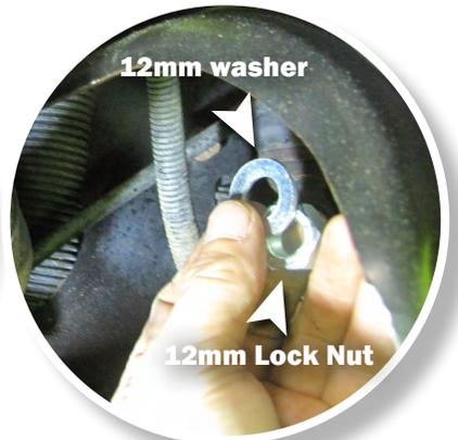
Secure the lower portion of the lift bracket with the 12x30mm bolt followed by a 12mm washer.
