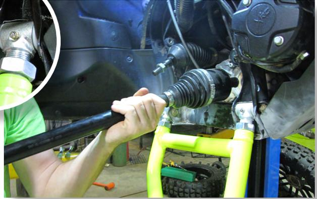
Install the new front axles into the differential.
