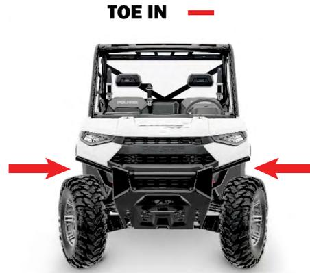
If the **FRONT OF THE WHEELS** are facing **IN**, adjust the tie rods **IN** or **REDUCE the length of the tie rod.**
