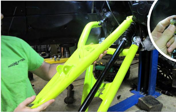
Secure the new upper control arm to the frame, using the factory hardware.
