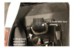
**STEP 3.** Locate the air box under the driver's side rear wheel well. Remove the air box lid by grabbing and rotating the handle counter-clockwise. Then remove the air filter by sliding the air filter out of the air box. Install KWT Flange (11) inside the airbox by aligning flange screws holes with the KWT Duct Adaptor (9) and tighten screws (10) at each corner of the KWT Flange. After the flange is installed, insert the air filter and close the airbox lid.
