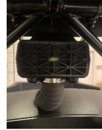
**STEP 2.** Loosen the four (4) hand screws in the recessed cups holding down the cargo bed. Remove cargo bed and set aside. Remove the intake cover by sliding the cover toward the rear of the vehicle. Set the cover on a sturdy surface.
