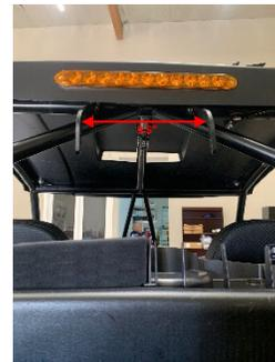
**STEP 6.** For upper roll bar installations use Step 5 with Metal Brackets (5) facing down. Install Particle Separator (1) onto the Metal Brackets (5) on the left and right-side using Screw (6) and Washer (4) and a 3/16" Hex Key to tighten. Washer **MUST** be between the Metal Bracket (5) and Particle Separator (1). If the washer is placed under the head of the Screw (6) the Particle Separator will rotate freely and may cause damage.
