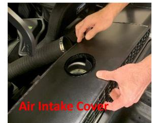
**STEP 4.** Uninstall the OEM rubber coupler from the air intake box and install the KWT coupler (8) on to the air intake box. Take the duct adapter (8) and place through the air intake cover hole and install onto the coupler (8). Tighten both hose clamps (2) on the top and bottom of the coupler.
