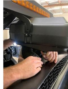
**STEP 7.** If necessary, cut excess off the Duct hose (9) with wire cutters for better fit. Insert a Hose Clamp (2) over one end of the Duct hose (9) and place over the Duct Adapter (8) and tighten. Insert a Hose Clamp (2) and the other end of the Duct hose (9) and place over the Particle Separator (1) intake and tighten with a Philips screwdriver, then fully Tighten screws on Metal brackets with 3/16" Hex Key.
