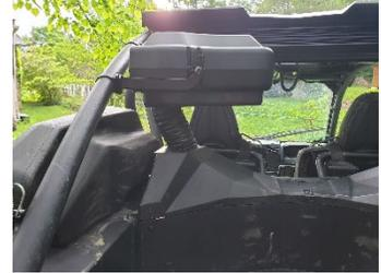
**STEP 2.** Remove push pins from plastic cover and remove cover. Loosen hose clamp from intake tube and remove intake tube from vehicle's air intake box and separate intake tube from side intake cover.
