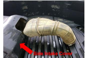
**STEP 3.** Remove push pins from the side intake and remove side intake.
