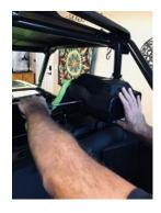
**STEP 5.** Measure Flexible Duct Hose (8) to Particle Separator (1) inlet, if necessary, cut excess off the Flexible Duct (8) with wire cutters for better fit. Insert the Hose Clamp (2) over the end of the Flexible Duct Hose (8) that is sticking out of the air intake panel. Place the Flexible Duct Hose (8) over the Particle Separator (1) intake and tighten Hose Clamp (2) with a Philips screwdriver. Once completed replace all side plastics back onto the vehicle.
