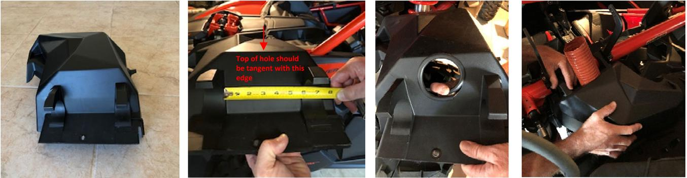
**STEP 5.** Install Particle Separator (1) onto the Metal Brackets (5) on the left and right-side using Screw (6) and Washer (4) and a 3/16" allen wrench to tighten. Washer **MUST** be between the Metal Bracket (5) and Particle Separator (1). If the washer is placed under the head of the Screw (6) the Particle Separator will rotate freely and may cause damage.
