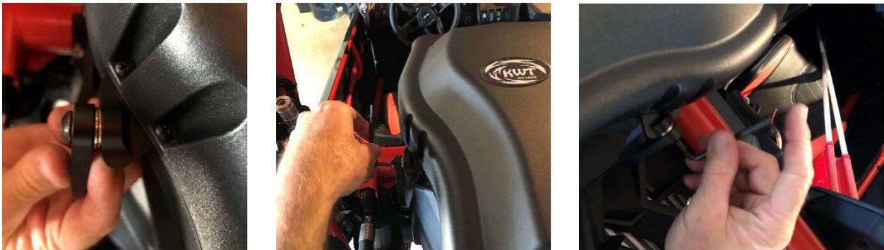
**STEP 6.** If necessary, cut excess off the Flexible Duct (9) with wire cutters for better fit. Insert the Hose Clamp (2) over the end of the Flexible Duct (9) that is sticking out of the Air Intake cover. Place the Flexible Duct (9) over the Particle Separator (1) intake and tighten with a Philips screwdriver.
