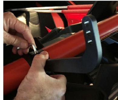
**STEP 3.** After Roll Bar Clamps (1) are installed, measure gap between the Metal Brackets (5) and set at 9.5 inches and tighten bolt. Insert the Duct Adapter (8) inside the vehicles air intake prefilter. Then install the vehicle air intake prefilter back into the vehicle. Place a Hose Clamp (2) over the Flexible Hose Duct (9) and insert onto the Duct Adapter (8) and tighten with Philips screwdriver.
