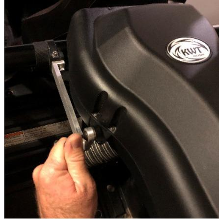
**STEP 7.** If necessary, cut excess off the Flexible Duct Hose (8) with wire cutters for better fit. Insert the Hose Clamp (2) over the end of the Flexible Duct Hose (8) that is sticking out of the Air Intake cover. Place the Flexible Duct Hose (8) over the Particle Separator (1) intake and tighten with a Philips screwdriver.
