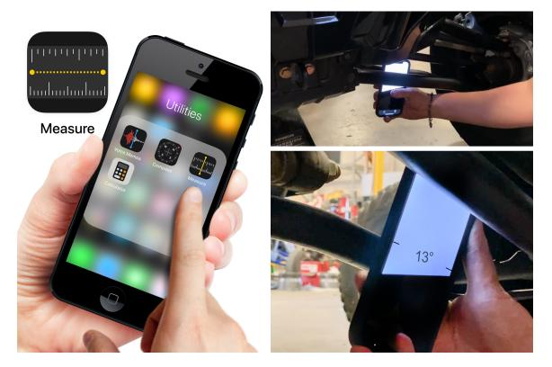
35. Your front and rear axles should measure to <u>12 - 13 degrees</u> (+ or - 1 degree). If your axle angle is less than 12 - 13 degrees then increase the preload, if it is more than 12 - 13 degrees then decrease the preload
