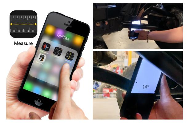
36. Your front and rear axles should measure to <u>14 degrees</u> (+ or - 1 degree). If your axle angle is less than 14 degrees then increase the preload, if it is more than 14 degrees then decrease the preload
