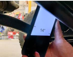
36. Your front and rear axles should measure to 14 degrees (+ or - 1 degree). If your axle angle is less than 14 degrees then increase the preload, if it is more than 14 degrees then decrease the preload
