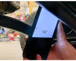
35. Your front and rear axles should measure to 14 degrees (+ or - 1 degree). If your axle angle is less than 14 degrees then increase the preload, if it is more than 14 degrees then decrease the preload0
