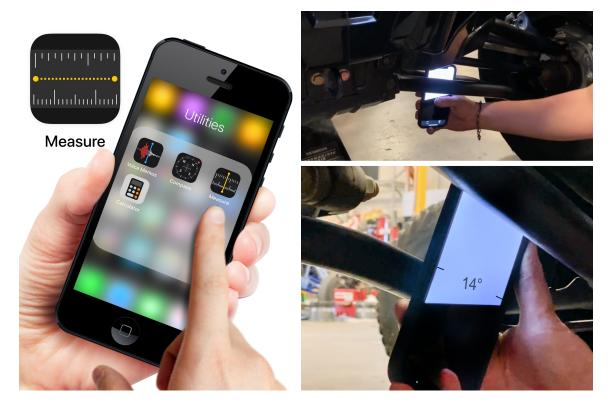
35. Your front and rear axles should measure to <u>14 degrees</u> (+ or - 1 degree). If your axle angle is less than **14 degrees** then increase the preload, if it is more than **14 degrees** then decrease the preload
