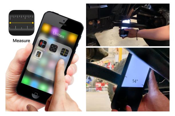
Your front and rear axles should measure to <u>14 degrees</u> (+ or - 1 degree). If your axle angle is less than 14 degrees then increase the preload, if it is more than 14 degrees then decrease the preload
