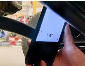
35. Your front and rear axles should measure to 14 degrees (+ or - 1 degree). If your axle angle is less than 14 degrees then increase the preload, if it is more than 14 degrees then decrease the preload
